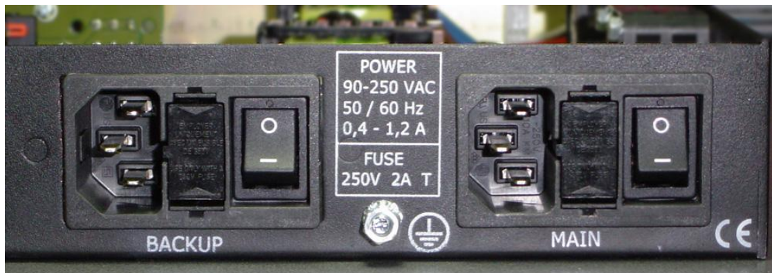
Rear view of main and redundant AC power supplies
